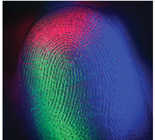
Illuminating the GelSight elastomer from three different directions allows the sensor to generate a 3-dimensional image.
